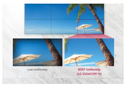
\* Uniformity among 13 points of the screen. Results based on in-house testing. Actual test results may differ depending on environment and measuring equipment.
