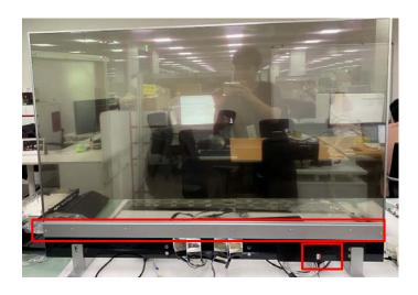
The FFC Cable & Touch PCB can easily be removed by hand and screw driver.
