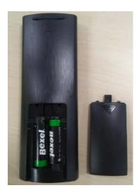
Batteries can easily be removed from the PCB Assembly once the back cover of product has been removed.
