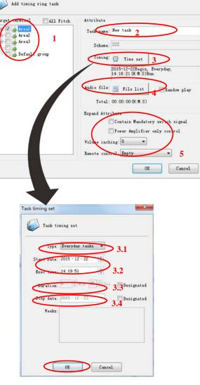
Fulfill the ring task parameters, press **[OK]** to exit the dialog box, the list will display the new added task, it will auto-execute at the assigned time, it also can use manual operation for special situation.
