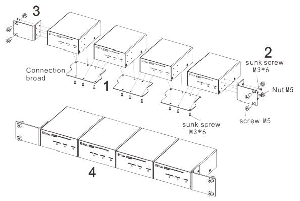
Using the half cabinet mounting bracket(MB-IP10B-BK) to fix the four devices as the mentioned method, then using length M5\*12 and above screw to install the devices in the suitable place.
