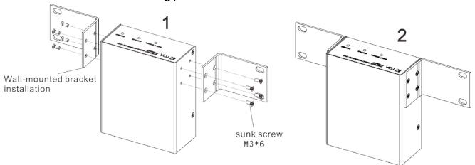
Using the countersunk head screw M3\*6 to fasten the two wall-mounted bracket in the two sides of the device, and then installing the device in a suitable position by screw(non standard) or expansion screw(non standard).
