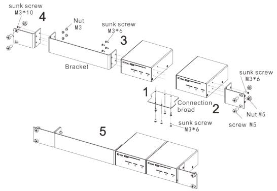
Using the half cabinet mounting bracket(MB-IP10B-BK) to fix the two devices as the mentioned method, then using length M5\*12 and above screw to install the devices in the suitable place.
