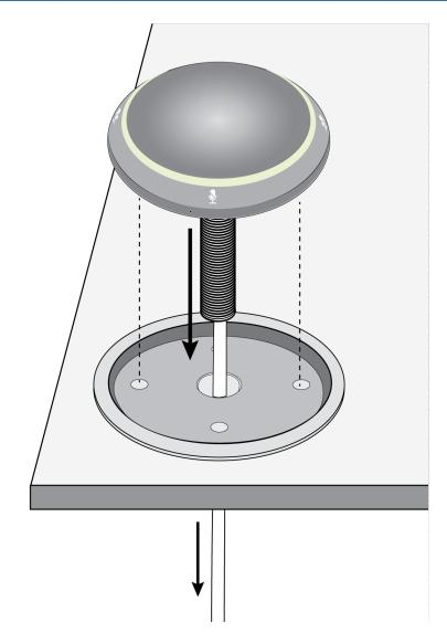
Place the bracket underneath the table, with the tube going through the hole. For thicker tables (≥ 55 mm), turn the bracket upside down for additional clearance.
