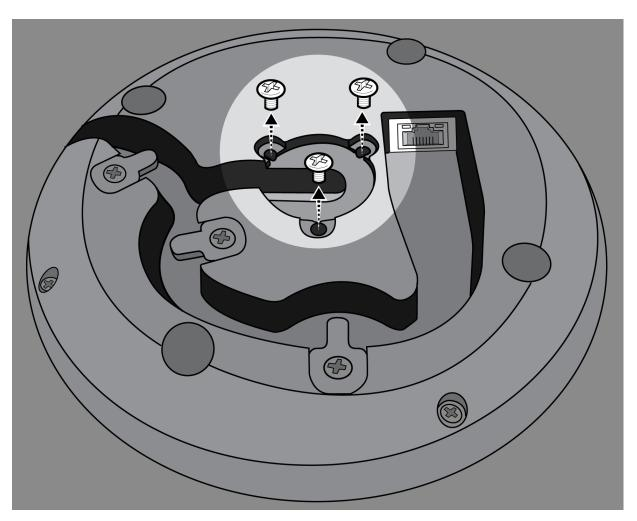
2. Plug a network cable into the microphone and guide it through the center exit path. When the cable is secured, guide it through the tube.
