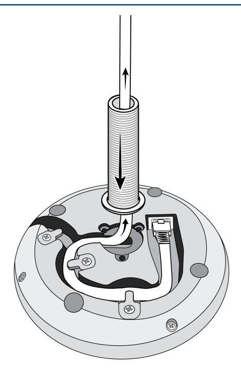
3. Align the tube into the recessed area in the center of the microphone. Install the 3 screws (removed in step 1) to secure the tube.
