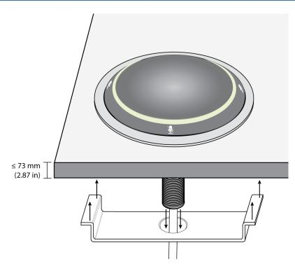
7. Guide the cable through the wing nut, and attach the wing nut onto the tube from underneath the table. Then, tighten the wing nut to secure the bracket against the table.
