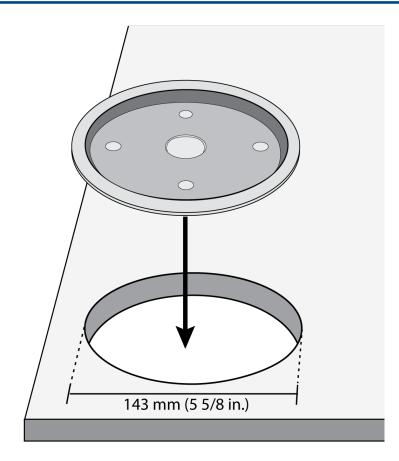
5. Guide the cable through the hole in the center of the tray. Then, place the tube through the hole in the table and gently press the microphone into the tray. Align the Shure logo on the microphone with the Shure logo on the tray. The four rubber feet on the bottom of the microphone fit into the four smaller holes in the tray.
